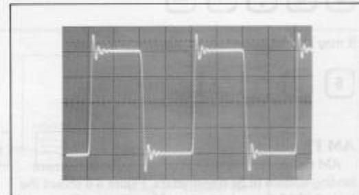
Figure 4-11. Demodulated 10 kHz FSK signal without >20 kHz low pass filter.
